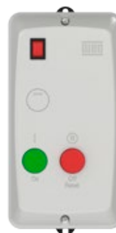
Chave Auto-OFF-Man (Auto=remoto/ Man=local) + Liga + Desliga/Reset
